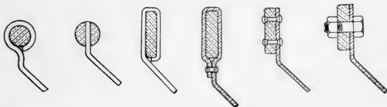
FIG. 403.—Methods of jointing Bars and Connectors.
